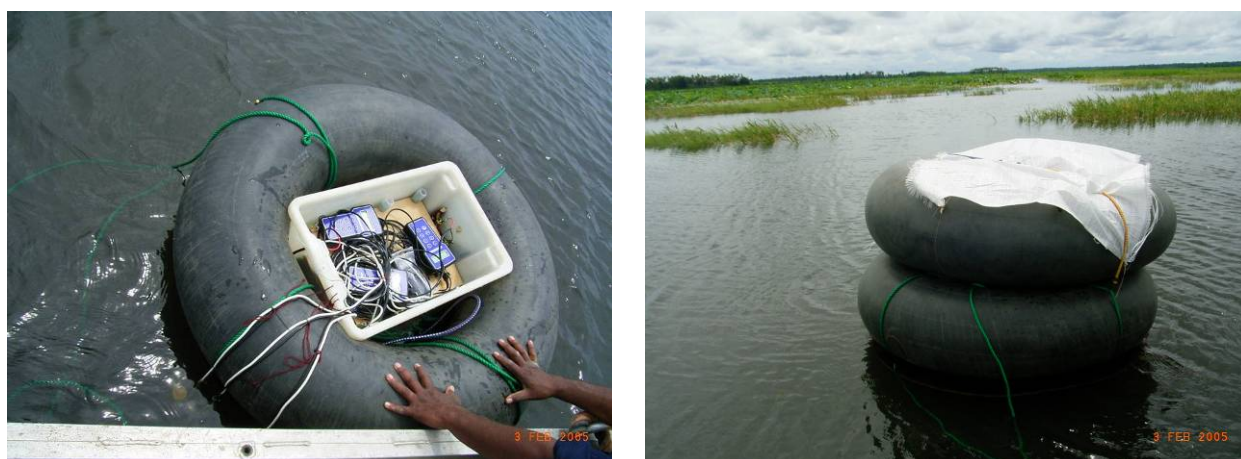
Plate 1. Anchored platform showing loggers in situ in a weather proof container without a lid (left). The cables to the three probes can be seen trailing over the side into the water. The complete unit, with shade cloth to protect the data loggers (right), in situ in Lake Daviumbu.
