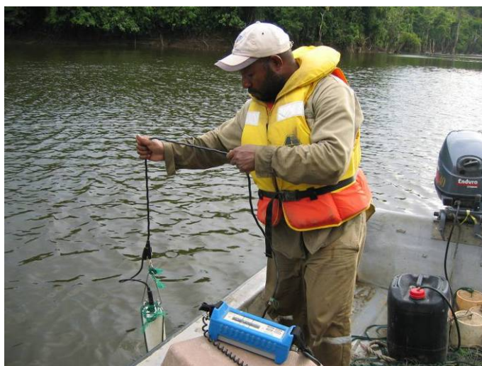
Plate 2. Hydrolab multiprobe in use.
